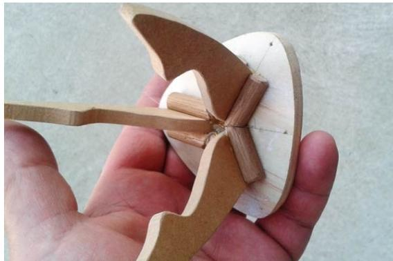
The fillets are made from 8mm dowel, shaved to make a quarter round, as shown in the photo above. You could use virtually anything that is handy.
