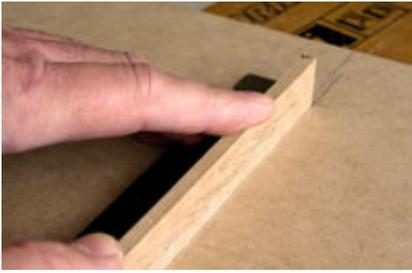
Step 4. It is important to cut the slots as accurately as possible for a good fit. Scribe one side with a sharp knife, use a scrap piece to measure then scribe the other side. Aim for a slot that is not too loose or too tight.
