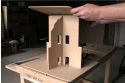
Step 7. Test fit the floors over the two walls. They should sit flat on all of the support steps. Once again, you might need to adjust the slots with sandpaper wrapped around a piece of scrap MDF.
