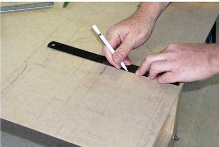
Step 1. Carefully mark out the board after studying the plans to see how everything fits together. A set of compasses are useful for marking out parallel lines. Shade the waste areas to be sure you cut on the right side of the pencil lines.
