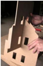
Step 6. Trial fitting of the two walls. If the slots are too tight, wrap sandpaper around a scrap piece to adjust the slots.
