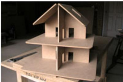
With all the pieces fitting together properly, round off all the edges with a sanding block.
