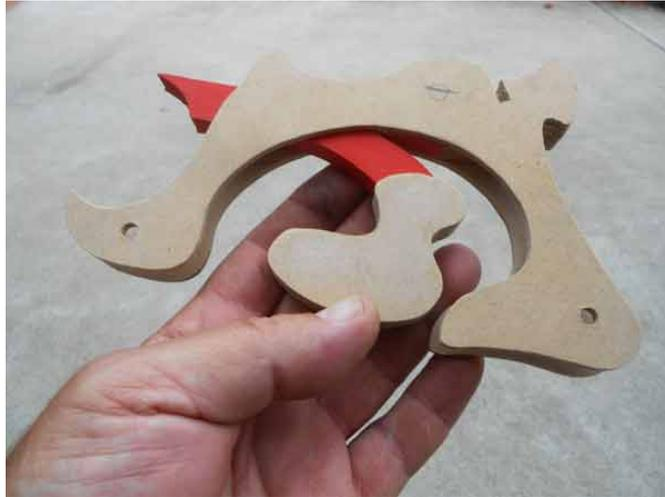
Showing the two outer parts are glued in place. Note that it is a good idea to insert the axles while the glue is setting – this will ensure that the parts are aligned.
