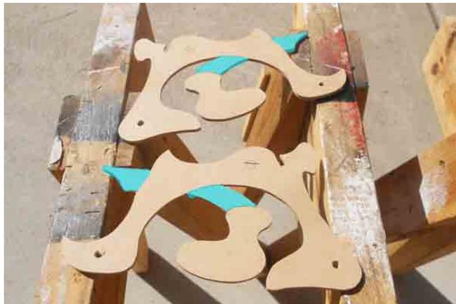
The shape is cut out, and the two outer sides are removed. The blue shading is the areas to be cut away.
