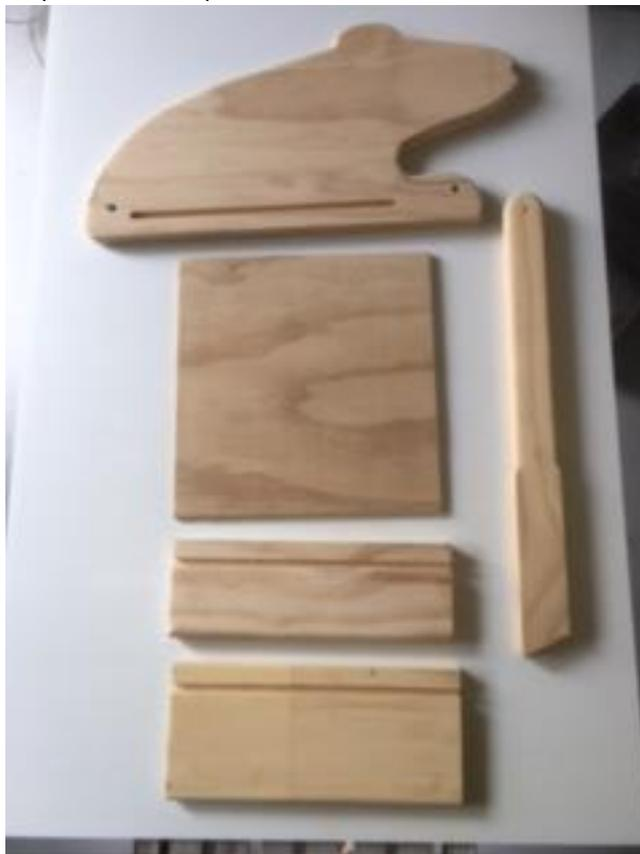
1. Using a 6mm router bit (i.e. thickness of the floor) cut 2 x slots 270mm long, 19mm from base of frog sides.
