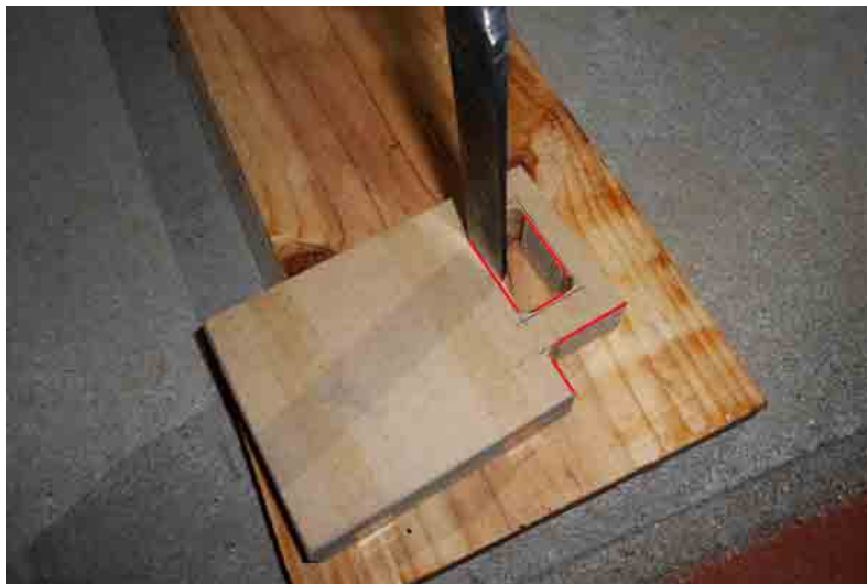
Photo 7: Cutting the windows
