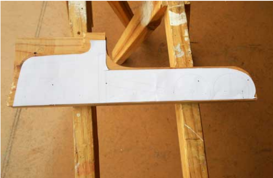
Step 1 Template attached to work-piece
